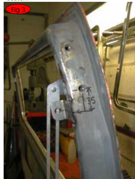
Centre the frame horizontally so that you have an even gap on the left and right of the frame. Mark exactly the ends of the hinge on your body. This allows you to open the frame to mark hole location.
