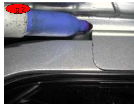
Centre the frame horizontally so that you have an even gap on the left and right of the frame. Mark exactly the ends of the hinge on your body. This allows you to open the frame to mark hole location.
